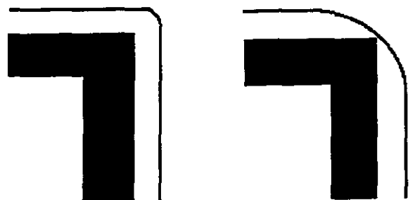
The effects of viscosity/thixotropy on edge coverage
